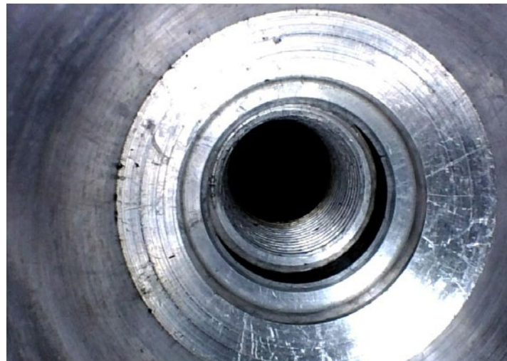
Photo above: Spark plug port inspection
